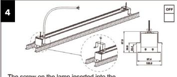
The screw on the lamp inserted into the T-BAR bracket and fixed with M5 wing nut
