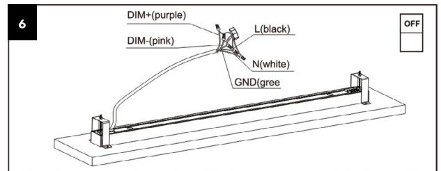
The dimming positive pole of the lamp is connected to the positive pole of the dimmer, and the dimming negative pole of the lamp is connected to the negative pole of the dimmer.
